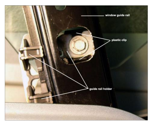
The tabs on the back of my plastic clip broke off and were not long enough to spread open and hold the window in place. Concequently, the window slipped off the plastic clip (with a thunk) and jammed the window in its track, causing the motor to stop.
