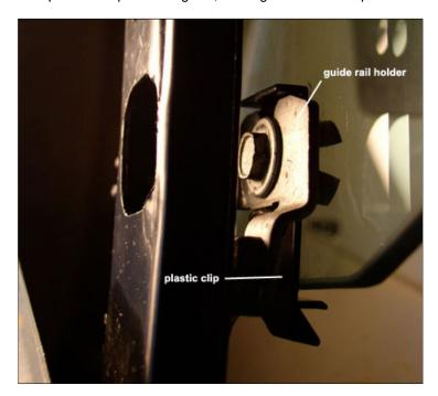
Inspect the window guide rail holder while you're in there. It also has a plastic element (connecting to the cable) which cracks over time due to the jerking motion of the motor. Mine's cracking. This is also the cause of our window problems, causing the cable to strip thru the holder, resulting in a jammed window. Unfortunately this part is not sold separately and must be purchased with the whole new window motor/track assembly.
