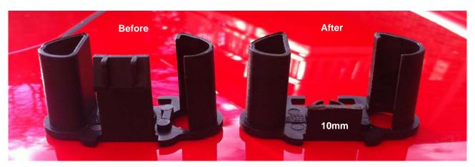
Next, take the two rear end caps and remove parts of the sheaf as shown so they slide all the way onto the bar.
