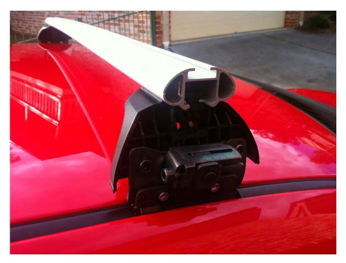
Now it's time to start modifying..... Grab the end cap guides and trim off the centre tab from two of them, leaving about 10mm on it. After playing around with the front, I figured you could have cut them off entirely, but it slips into the bar nicely this way.
