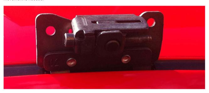
Then, mount the foot pack – RT753 (loosely) to the fitting kit. I say loosely, as the bar clamp in the centre tightens onto the bar as you tighten the allen screws connecting the two assys. No modification to the rear foot pack is required.
