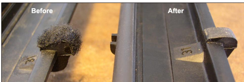
**8)** Re-install modified rain gutter in reverse order, then install modified ceiling liner with handle, and then roof panel. Now enjoy reliable sunroof operation!
