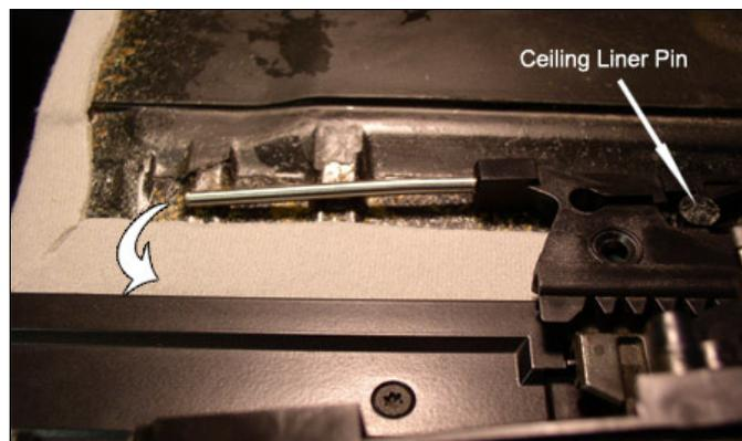
3) Using T-25 torx, remove the 3 now-visible sunroof panel screws on inside of each lifting gate arm. Lift panel out; set aside.
