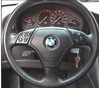
Note these two wheels offer customizable button block options. For instance, telephone buttons are optional, while wheel A may include either wheel heater or HVAC recirculation button (unusable with 8-series). Wheel B has no heat option but offers button covers. (Wheel C has no options.) Therefore, for example, wheel B could be configured with radio buttons only. For button block details, see RealOEM [wheel A](#), [wheel B\(1\)](#), [wheel B\(2\)](#), and [wheel B\(3\)](#).
