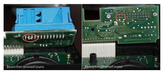
Removing the front panel controller requires console trim removal and disassembly of the controller. An alternative which does not require controller disassembly is splicing wire 11 and 12 together.
