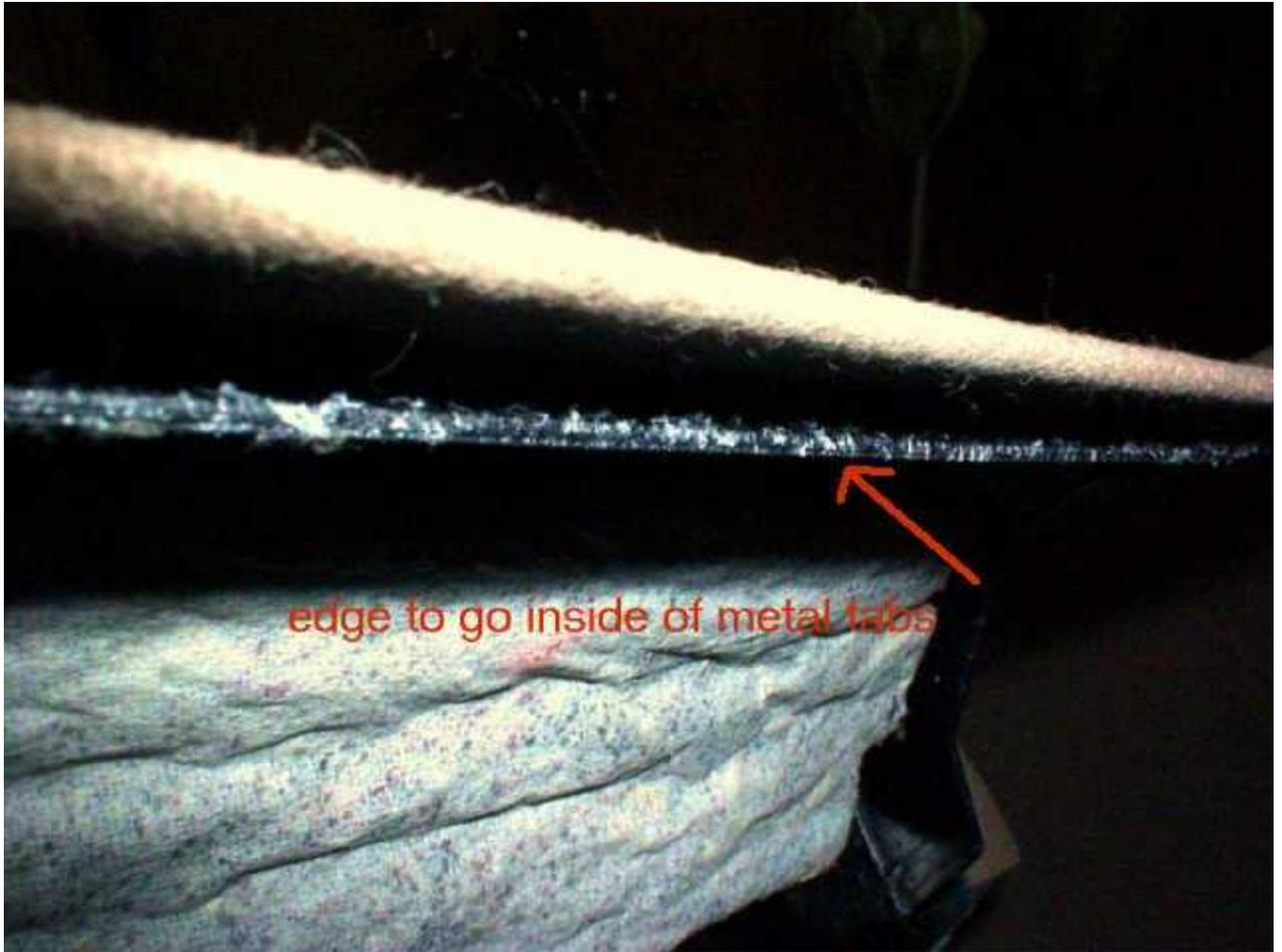
Engage the c-pillar covers by squeezing them and inserting the edge clips (see picture) and pushing the 4 plastic tabs into the 4 rectangular clip holes. I did this WITHOUT using the metal clips since it is held in place by tension after it is no longer being squeezed, and by foregoing the metal clips I should be able to remove the c-pillar covers in the future without breaking the tabs. Replace the c-pillar lights.
