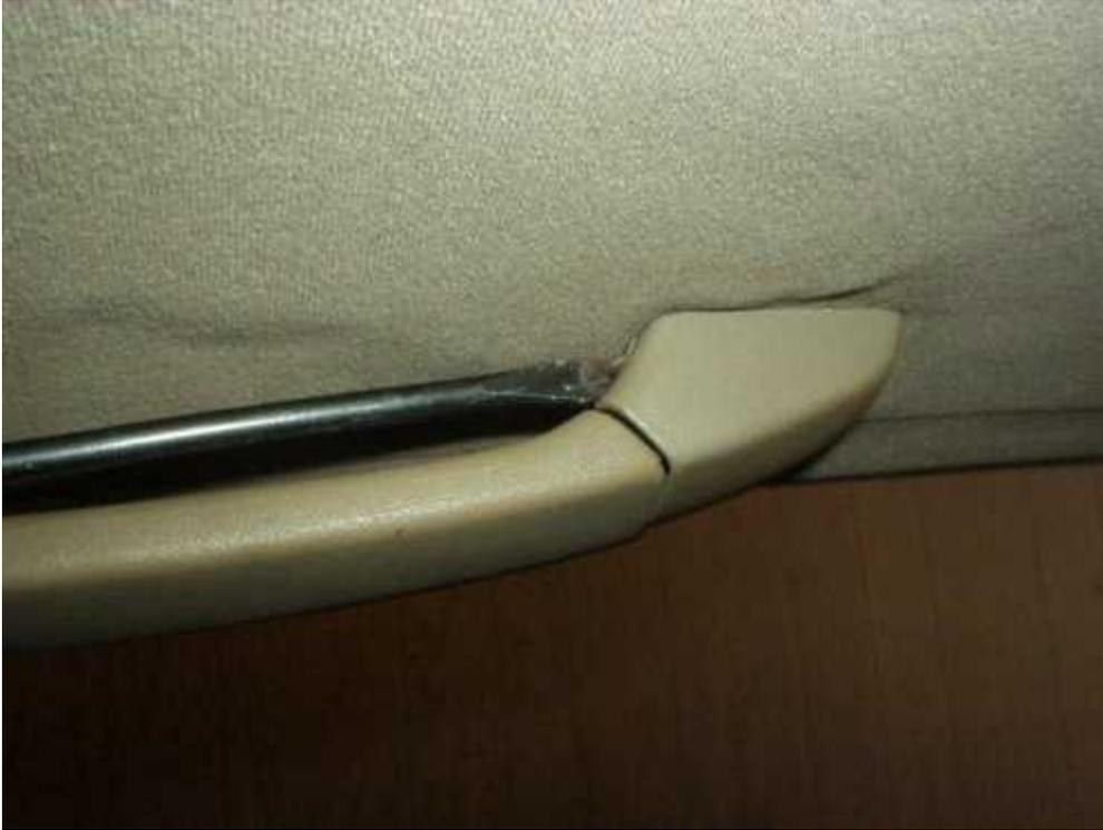
Remove the visor holder mounts, torx screws, be careful pulling out since there is a wire attached to each. Remove the visor swivel mounts, they also have a wire attached.
