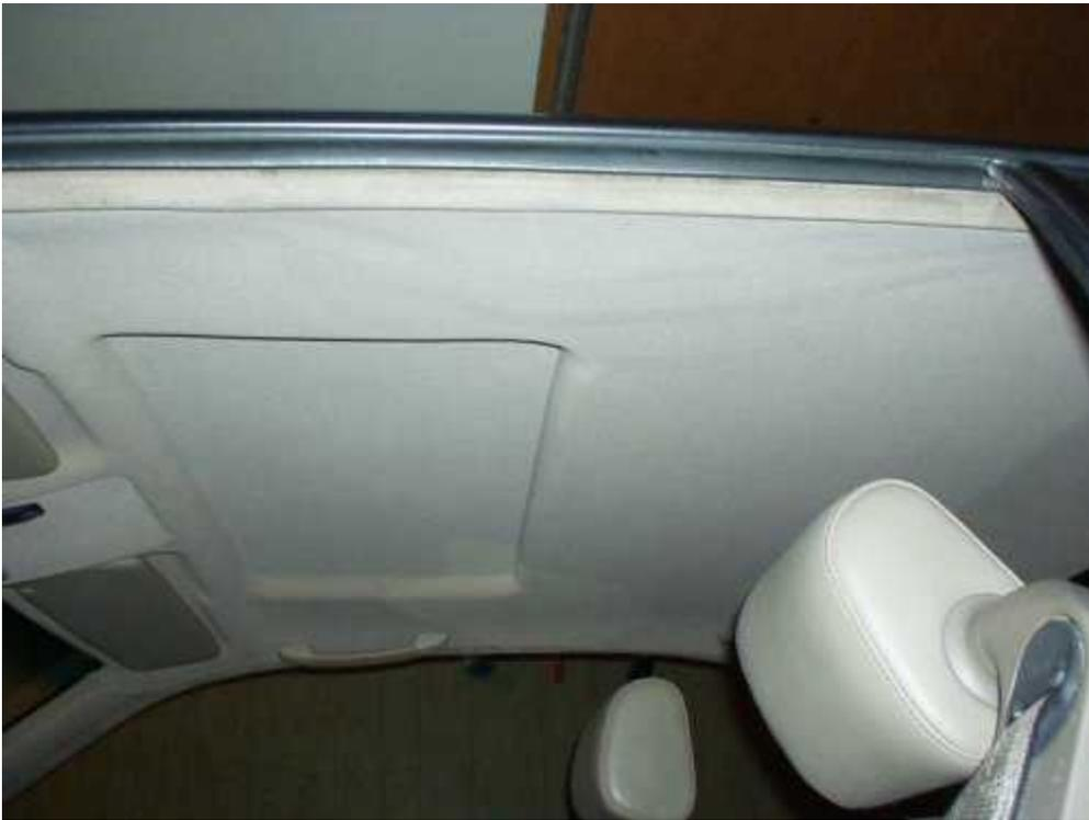
The “wrinkles” you see above the driver’s side were impressions from the protective plastic sheet pressed against the fabric during shipping, and have disappeared since install.
