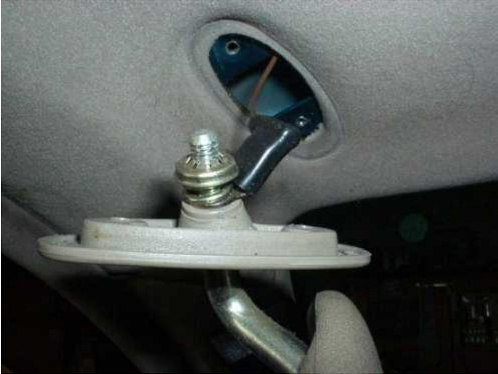
Remove the visor light panel by working out of headliner with fingernails or putty knife. Socket for connector is facing you on reinstallation.
