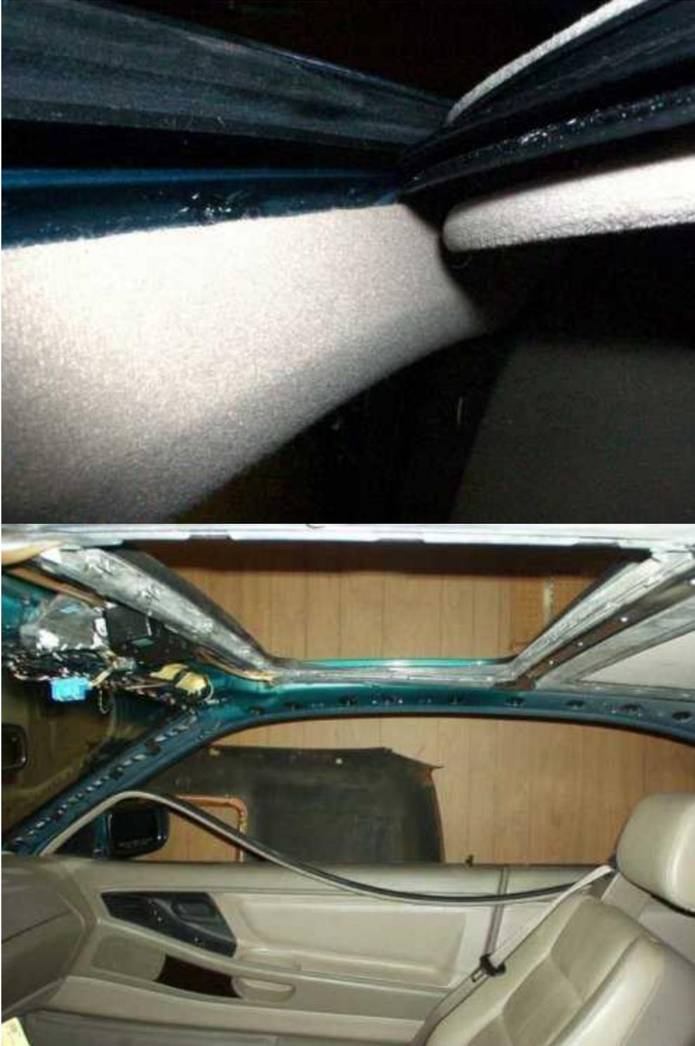
With all windows open, pull headliner down and free it to where the only thing holding it in is the rear lip. Sitting in car, grasp it at rear of sunroof opening and push it backwards to disengage rear lip. Then have helper maneuver it out of the car through the open windows. Set aside in a safe place, especially if you are going to recover the sunroof sliding felt panel. I used a product called SOF SOLE
