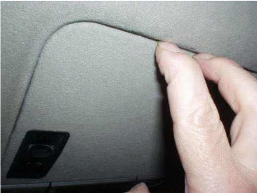
Remove passenger "Oh Sh\*t" handle by inserting a flat blade screwdriver at mount seam at either end of handle and pushing mount cover outwards and pulling cover off. Then unscrew Phillips screws. Work handle out of headliner and set aside.
