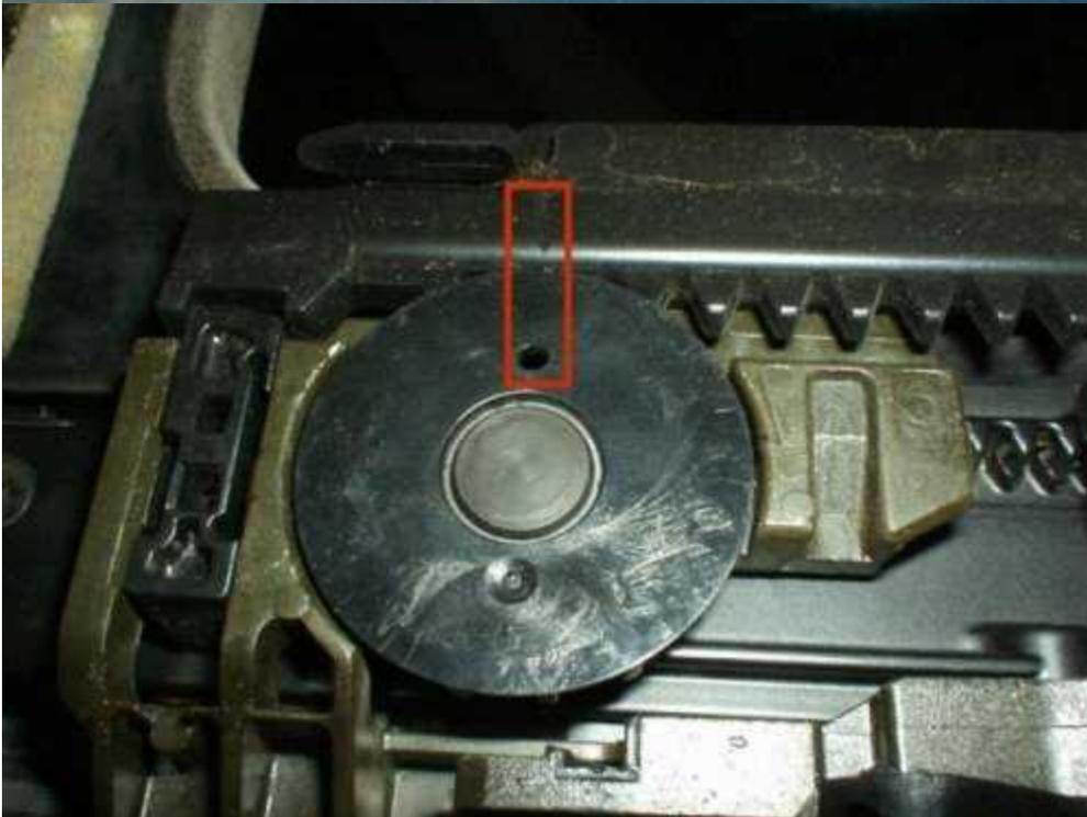
Insert the inverted metal “T” under the metal spring clip on the sunroof bracket, and make sure the metal sunroof screw holes are lined up with the bracket screw
