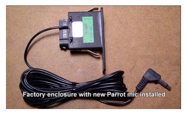
TIP: Splice a common wiring connector into mic wire (behind mic) to allow for enclosure detachment, in case the center console needs to be removed in the future.
