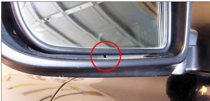
2) With mirror loose, disconnect heater wire connections and set mirror aside. See image below:
