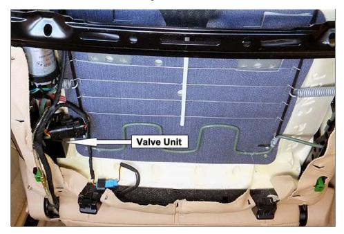
The valve unit will be partially hidden by various other wires and connectors; unplug and move them out of the way.
