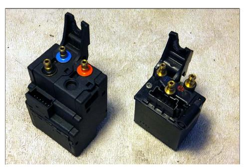
• (1) Lumbar Valve Unit, p/n 67 66 8 385 632 list: \$129, used: about \$25 (samples shown above)
