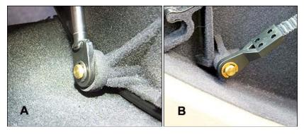
5) Similarly, remove circlip from right side extension strap and remove it from its pivot arm. See image above, panel B (see also #21 diagram A).
