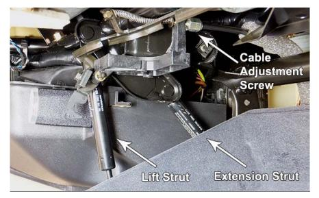
This screw adjusts the cable's sheath. Turning the screw back (towards front of car) applies more tension to handle, and vice versa. The other end of sheath must be correctly installed (from #1 above) for this to work. Typically, little or no cable adjustment will be needed.
