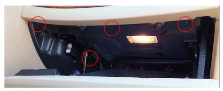
Drop front of cover and unplug connectors for glovebox light and light switch. Set cover aside.
