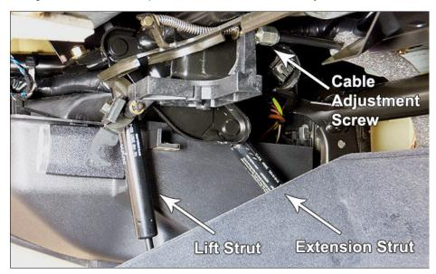
This screw adjusts the cable's sheath. Turning the screw back (towards front of car) applies more tension to handle, and vice versa. The other end of sheath must be correctly installed (from #1 above) for this to work. Typically, little or no cable adjustment will be needed.
