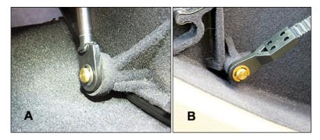
**5)** Similarly, remove circlip from right side extension strap and remove it from its pivot arm. See image above, panel B (see also #21 diagram A).
