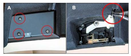
3) Using needle-nose pliers or similar tool, disconnect cable end from handle mechanism and extract cable from its channel on the lower left side of the glovebox. See image above, panel B.
