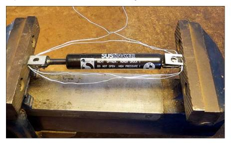
3) Remove compressed extension strut from vise and install onto glovebox swing frame.
