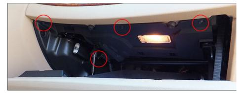
Drop front of cover and unplug connectors for glovebox light and light switch. Set cover aside.
