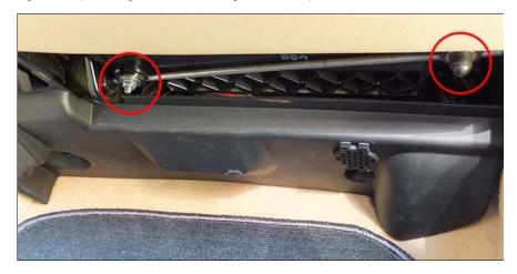
2) Open glovebox and remove the three (3) screws on the left which connect the handle cover to the handle. Remove cover along with screws and spacers. See image below, panel A (#7 and #8 in diagram A).
