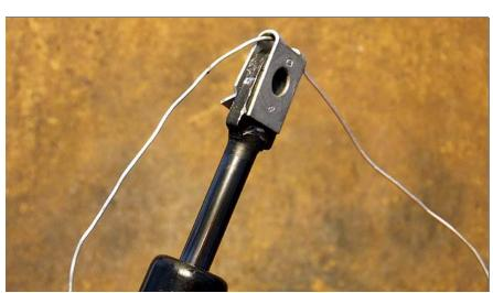
2) Place extension strut in a bench vise and compress approximately one inch. Draw wire tight by twisting with pliers or similar tool. This will hold strut in compressed state when removed from vise. See image below:
