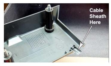
This will provide constant tension on the handle mechanism and returns the handle to "closed" position after being released. A slight tug on the cable after cover installation will confirm cable sheath is correctly positioned. Then, tuck cable sheath into slot along left side of glovebox for a clean install.
