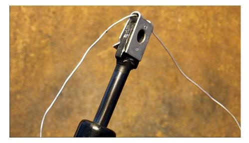
2) Place extension strut in a bench vise and compress approximately one inch. Draw wire tight by twisting with pliers or similar tool. This will hold strut in compressed state when removed from vise. See image below:
