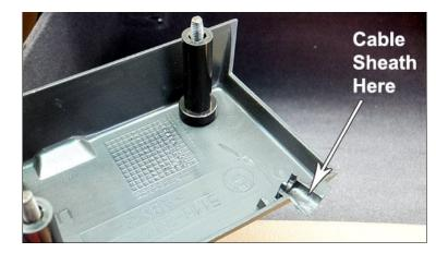
This will provide constant tension on the handle mechanism and return the handle to "closed" position after being released. A slight tug on the cable after cover installation will confirm cable sheath is correctly positioned. Then, tuck cable sheath into slot along left side of glovebox for a clean install.
