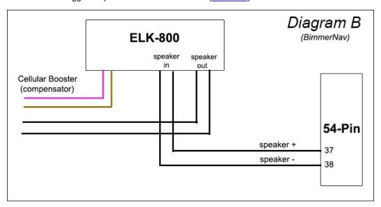
Reference the diagram printed on the amp's label for connections at the ELK-800. Strip 1/4" off the ends of each wire and secure them into the terminals of the amp by turning the small screw atop each respective binding post.
