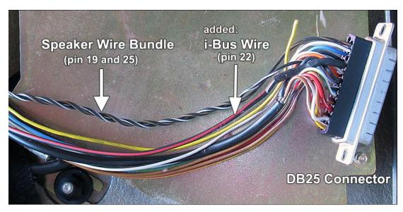
3) With the ELK-800 securely mounted in its location, snip the needed wires of the DB25 bundle in the most convenient place for access to the amp's terminals, according to this schematic:
