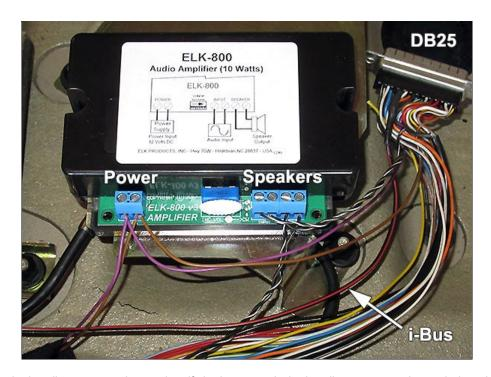
**5)** Re-wrap the DB25 wire bundle as appropriate and verify both amp and wire bundle are secure. Image below shows an installation in a '99 528iT, with both TCU and ELK-800 secured to mounting boards atop existing factory brackets.
