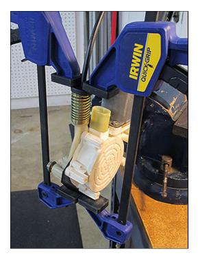
Otherwise use a helper to hold the spring in a compressed state while the repair is completed. Be sure to guide cable into spool housing as spring is compressed.
