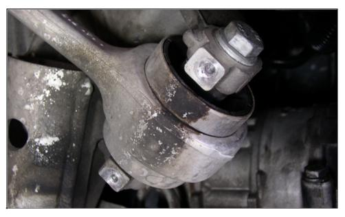
Above, notice how the stock bushing's fluid has leaked and stained the underside of the bushing and control arm. This confirms a failed bushing. (Meyle HD bushings are solid and contain no fluid.)
