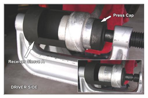
Begin by placing Press Cap on outside (front) of bushing, and Receiver Sleeve A on opposite end of C-clamp. A helping pair of hands will make this easier (or hold the C-clamp in place with your shoe while positioning the sleeve with your hands). Hand tighten jack screw to hold "the stack" in place.
