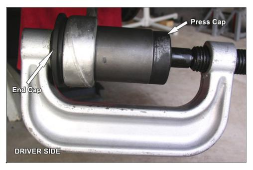
Grease jack screw liberally. Screw will become warm to the touch from friction of applied torque. You will soon notice the greater force required to press in new bushings versus removing the old.
