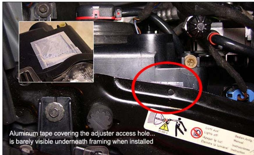
Aluminum tape covering the adjuster access hole... is barely visible underneath framing when installed
