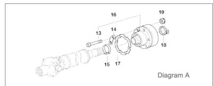
NOTE: Gasket (part #17) is erroneously shown to install forward of the CV joint; it actually installs behind it. New CV joints come with new bolts (part #13) and washers (part #14) but not nuts (part #19), so these will have to be re-used. New CV joint part numbers vary by model and year but look practically identical (see <u>ReaIOEM.com</u> for part numbers). Their replacement procedures are the same.
