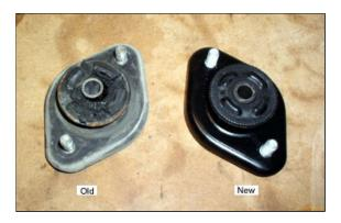
For reasons unknown, the E46 convertible shock mounts are reputed to be better than stock E36 mounts - and cheaper (p/n above). You'll need two new gaskets as well (p/n above).
