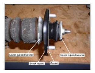
**10)** Install new shock assembly in reverse order. Tighten lower mounting bolt to 77 Nm (57 ft-lb). See Bentley service manual page 330-4 for other torque specs or just use a solid "snug" feel. Don't forget to pull rubber protective cap completely over upper shock mount once it's back in.
