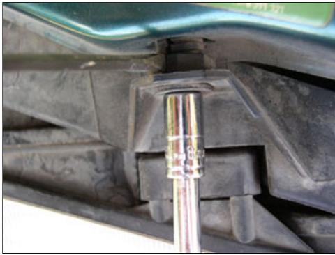
**2)** Using an extension bar, remove the remaining left and right 8mm screws, located behind the lens. You'll need a flashlight to see 'em. See images below.
