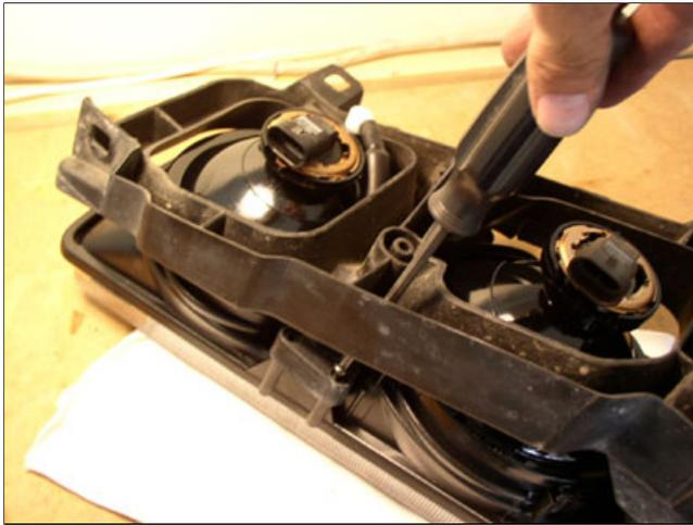
**6)** Finish installation of new assembly in reverse order. When complete, verify headlight aim and function. I used my closed garage door to project light onto. Consider protective lens covers on your new investment, too.
